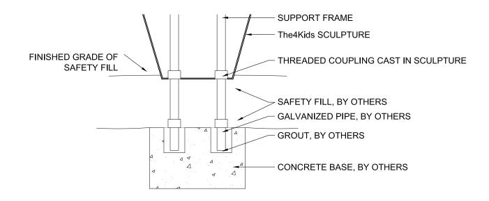
ADJUSTABLE METAL FOOTING IN CONCRETE PAD
